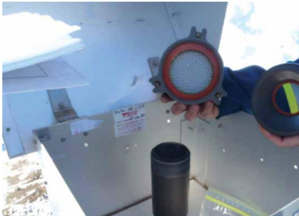
Figure 8 – Components of high volume sampler used to collect PAH samples.
