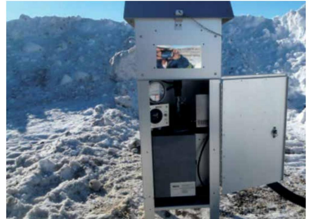
Figure 9 – Inside view of high volume sampler.
