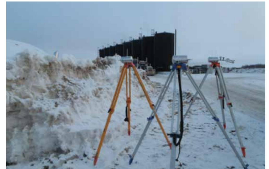
Figure 5 - View northeast of triplicate VOC samples 50 m downwind of tanks on pad 02-01.
