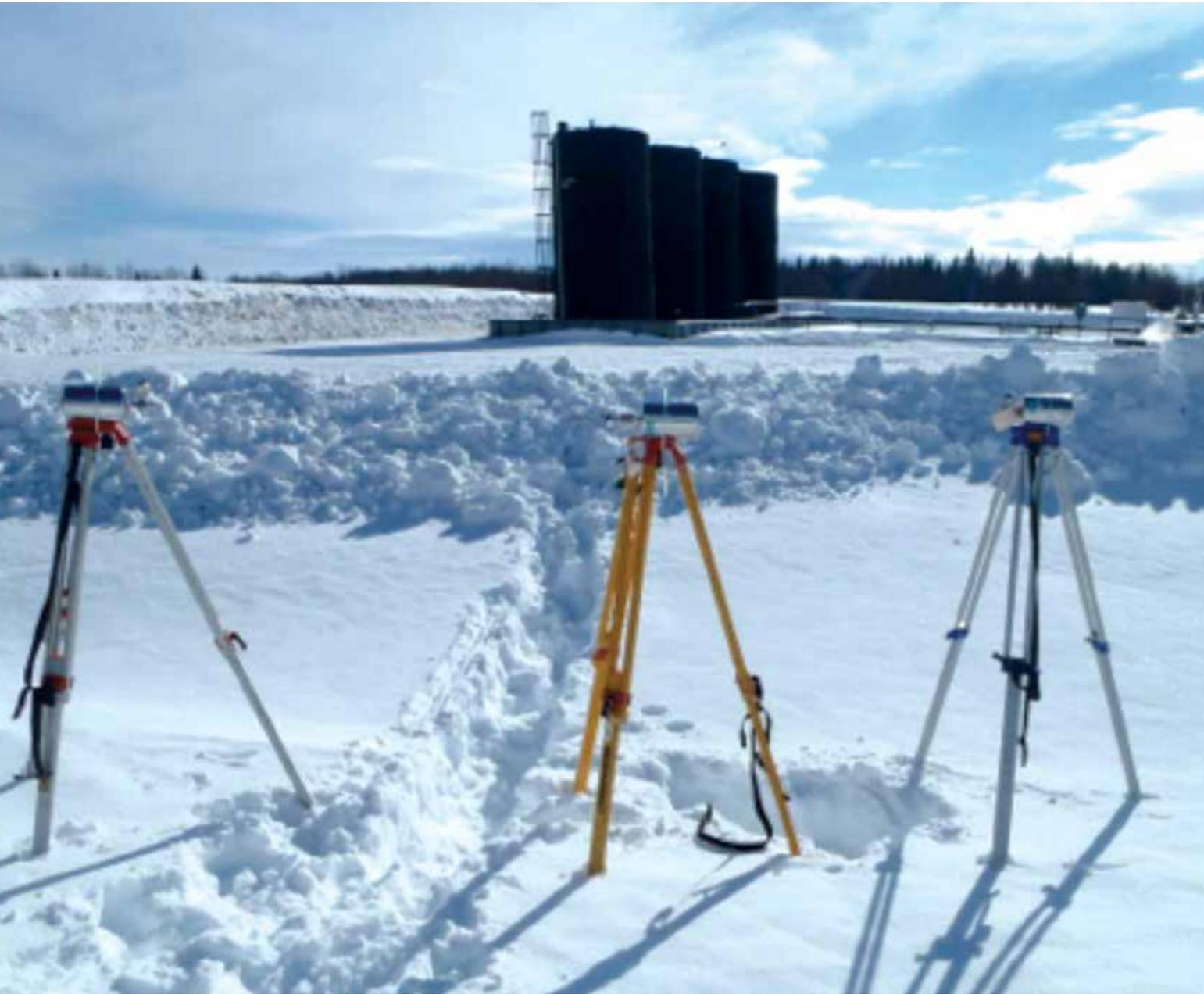
Figure 4 - View south of triplicate RSC samples 50 m downwind of tanks on pad 08-21.
